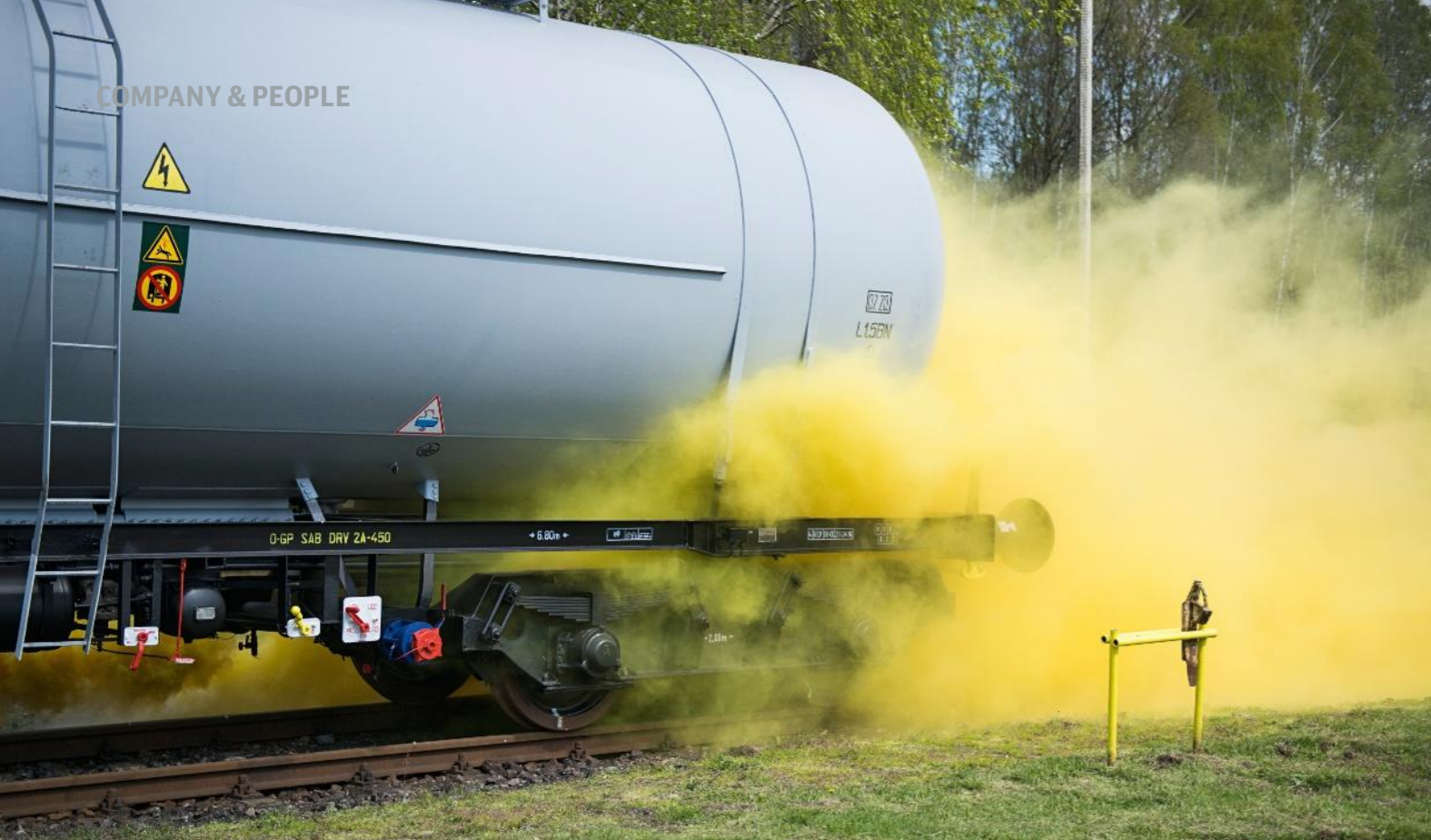
URGENT ASSIGNMENT: Dealing with a leak in a sulphuric acid tank wagon.
